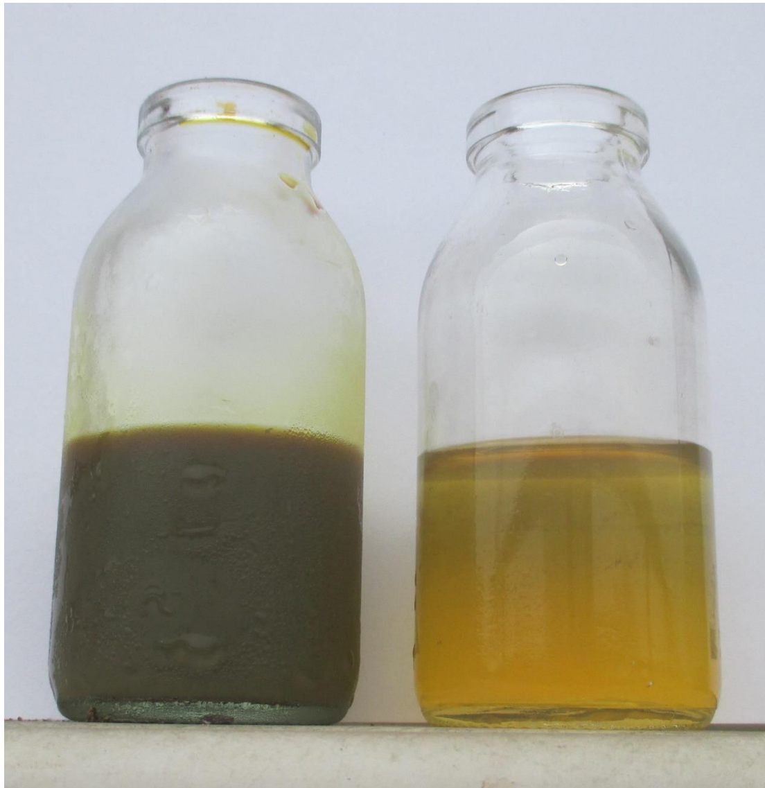
Fig 1 Left: yellow brown viscous non-transparent liquid of 500 ppm nano colloidal Silver, with yellow color on a container wall in shaking . Right: 50 fold-diluted solution (10 ppm nano colloidal Silver) is shine yellow.
